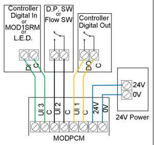
4, Connect the MODPCM motor side as shown
