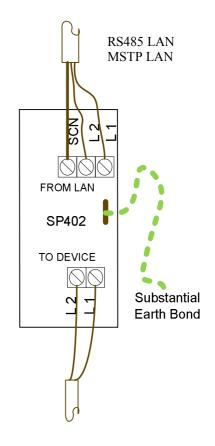
The level of protection is dependant on the module having a substantial earth bond to a true earth point. Keep the length of cable to the device to about 400 to 500mm.
